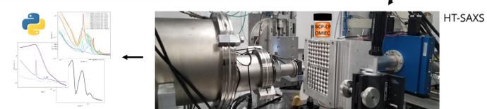
Figure 7. High-throughput small angle x-ray scattering (HT-SAXS)
